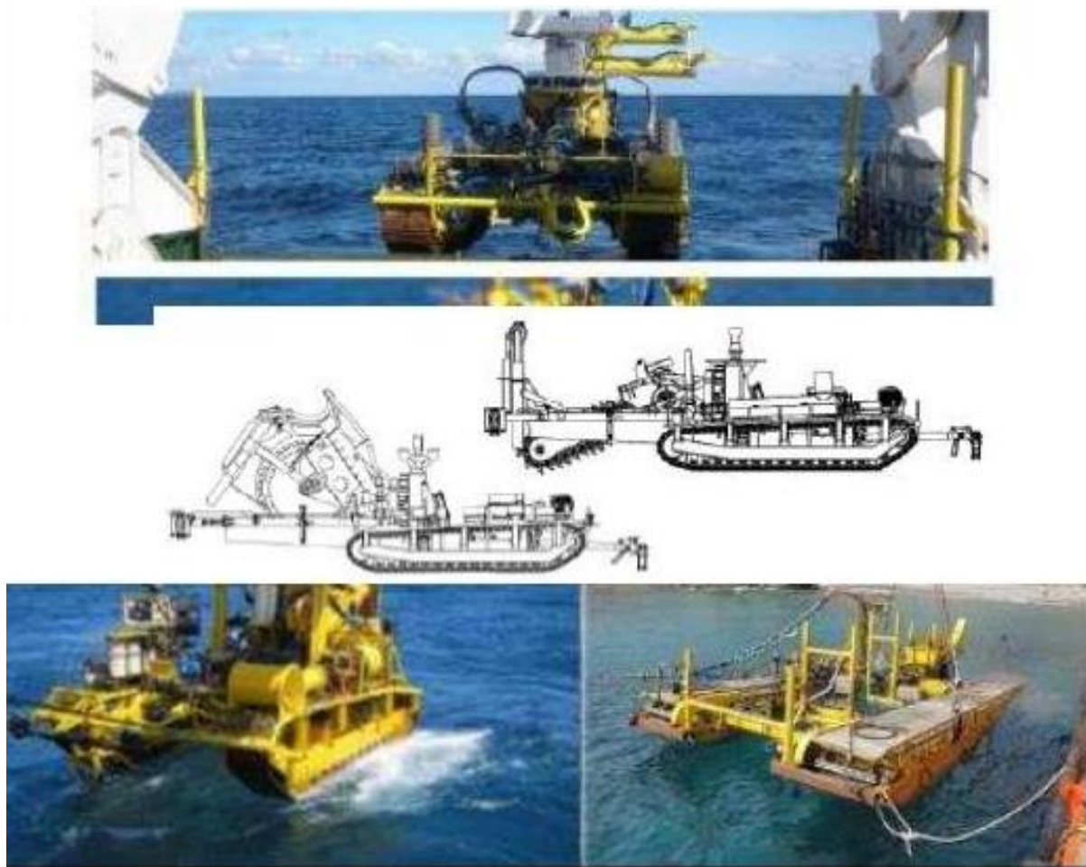
Figure 5.23: Conventional trenching machine
