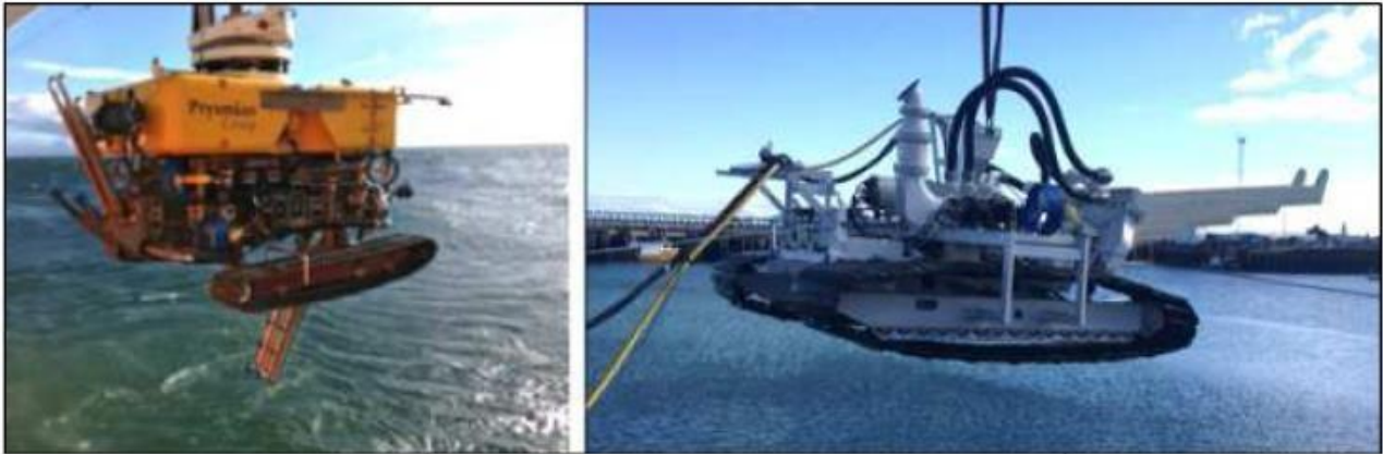
Figure 5.20: Tracked jetting machine
