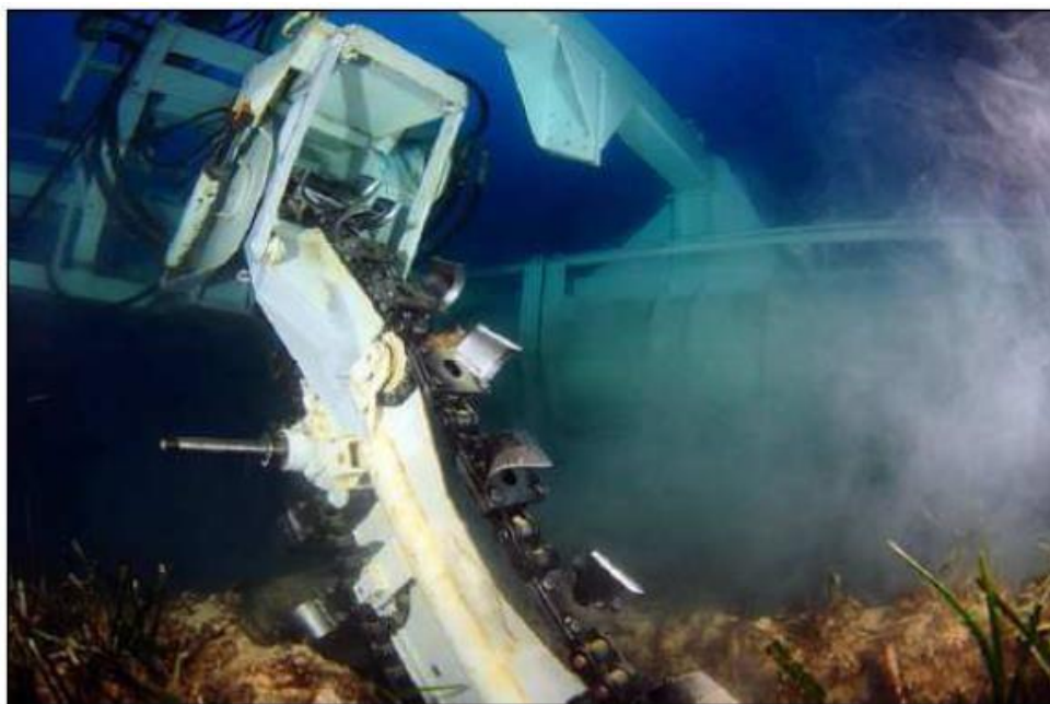
Figure 5.24: Cutting tool for trenching machine
