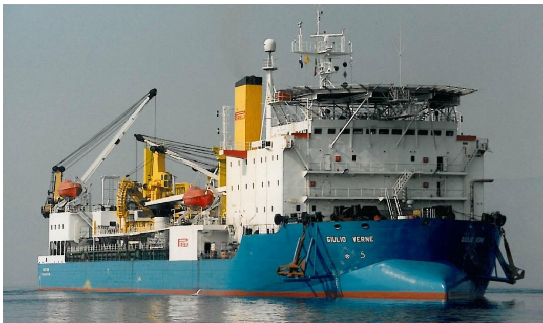
Figure 5.16: Cable laying vessel Giulio Verne
