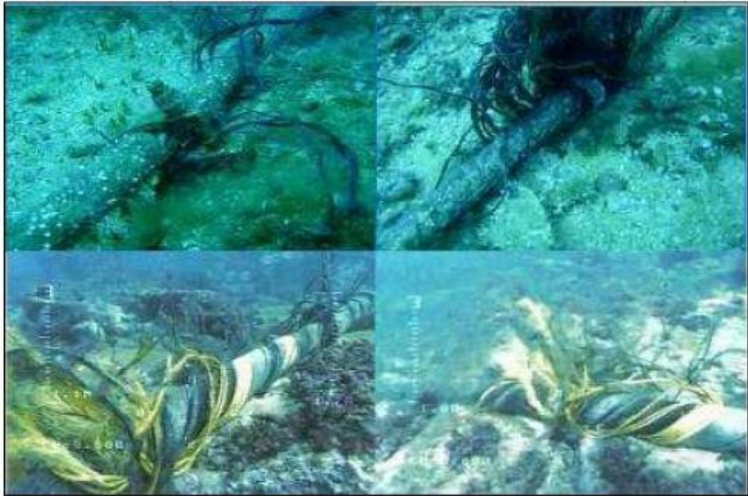
Figure 5.18: Unprotected undersea cables damaged by human activity
